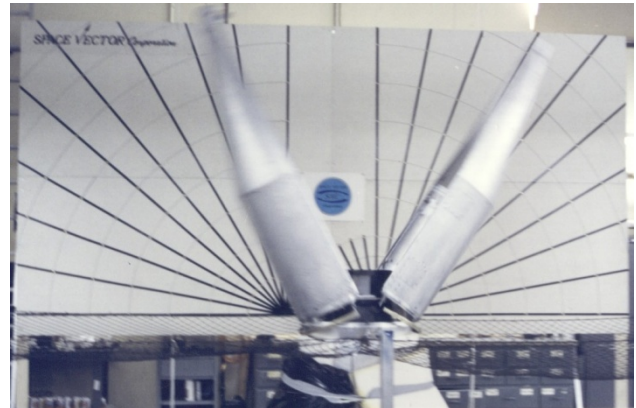
Nose Fairing Deployment Test at Space Vector
