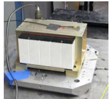
7 Ah Battery during RV Qualification Testing (shown in ruggedized horizontal restraint)
