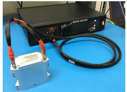
Batteries and Cells tested to RCC 319-14 with Charger/Analyzer 500451
